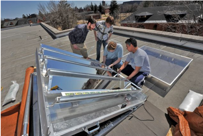
Fig. 10. Single-axis solar louver tracking design with 3M brand Cool Mirror (photo courtesy of Lake Superior State University).
