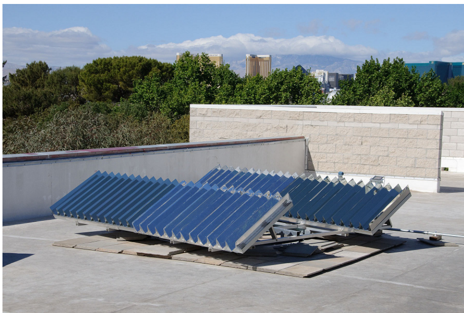
Fig. 6. Single Axis LCPV design with JX Crystal design using 3M Cool Mirror.
